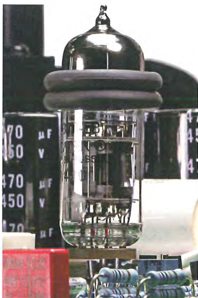
A 6H30 driver double triode, well known for ruggedness combined with good sound. It has anti-microphony damping rings on here.
